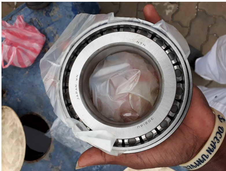
New NTN rudder bearings
