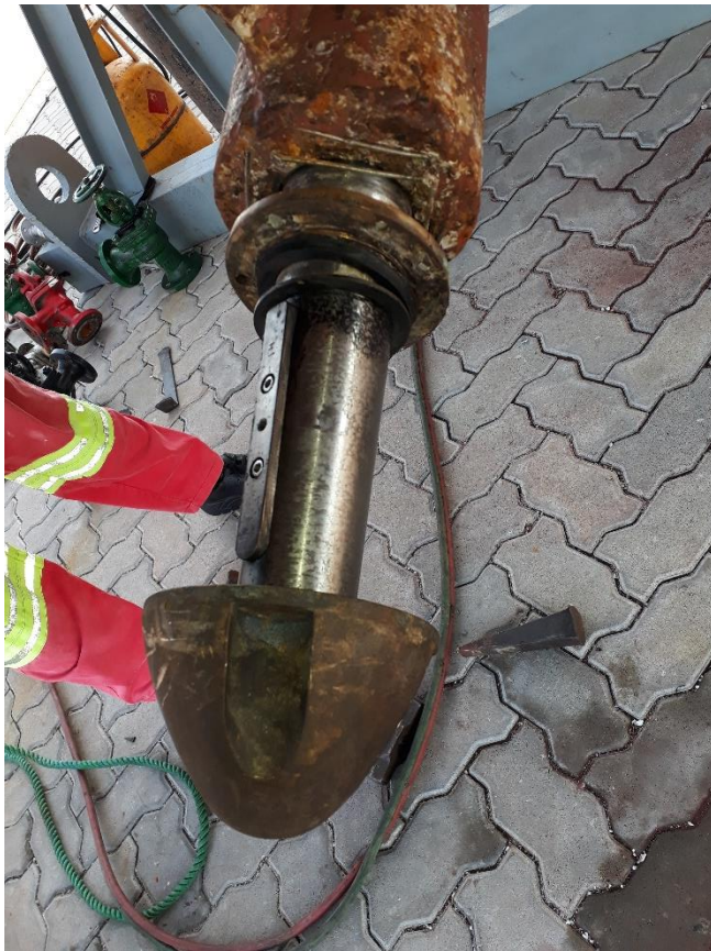
P side SS allon bolt head damage
