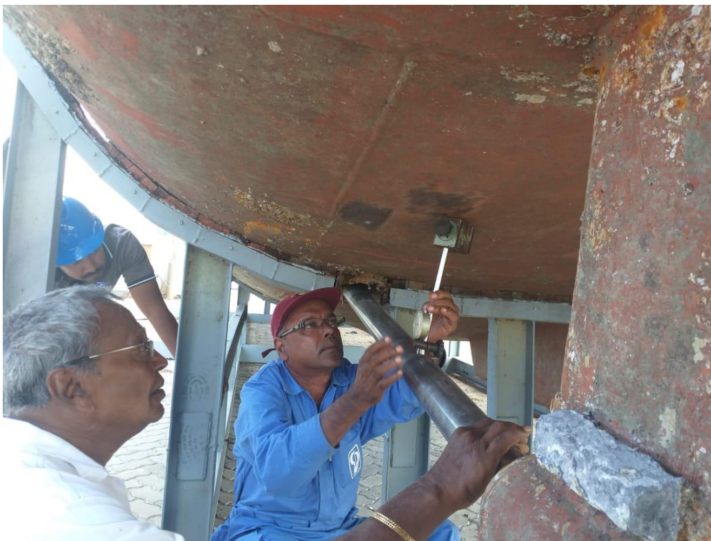
Shaft alignment checking by dial gauge
